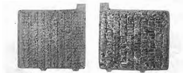
OVERCHARGED NEGATIVE & POSITIVE PLATES
